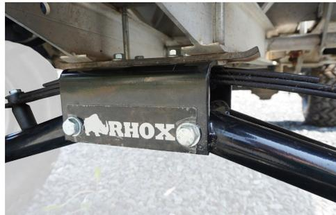
10. Install (1) 1/4-20 x .5" Hex Head Bolt and (1) 1/4-20 Nylock Nut onto the centering plate. Place the centering plate between the original shock mounting plate and the leaf spring mounting perch on the bottom of the axle. The 1/4-20 bolt head and nut will fit into the center hole of the spring perch and original shock mounting plate to aid in alignment of the riser block and mounting plates.
