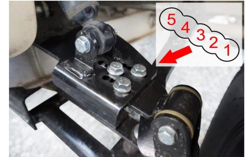
4. Once camber and toe adjustments are finalized and set, tighten all hardware and jam nuts.
