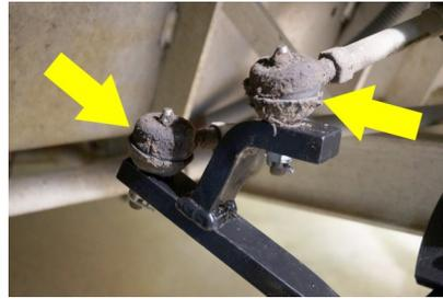
Reinsert the safety pins after the tie rod ends are seated properly.
