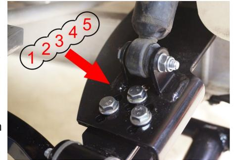
There are (5) adjustable camber positions. To start, it is recommended to use the second position from the outside of the cart. Final adjustments can be made once all tires are installed.
