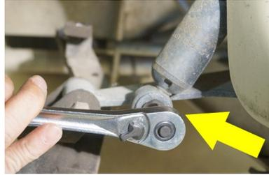
13. Disconnect the lower portion of the A-Arms from the spindles and discard hardware. Disconnect the upper portion of the A-Arms from the frame. Discard the A-Arms but retain the hardware and the A-plate straps (blue).
