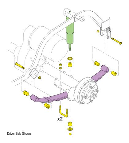
12. Carefully lower the rear axle away from the chassis with the jack. The jack stands will remain in place to support the chassis.
