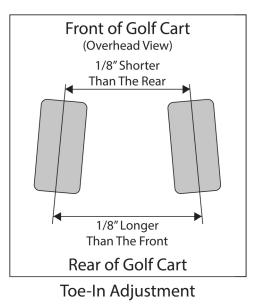
4. Once the toe adjustments are finalized and set, tighten the jam nuts.
