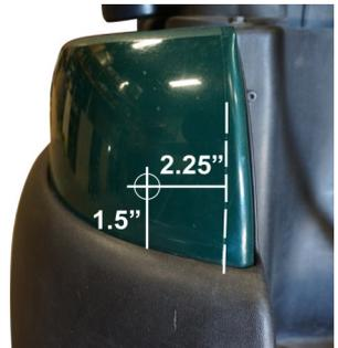
3. Electric carts 2004-2008.5 and gas carts: reach inside the holes of the rear body and pull the taillight connectors through the holes.
