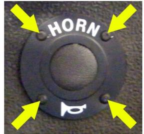
6. Locate the covered horn button connectors on the LGT-696 sub-harness and carefully remove the cover with a utility knife.
