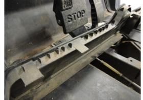
7. Feed the 12-pin connector and brake light wires on the LGT-396 harness from the battery compartment through the through-hole where the main harness runs to the front of the cart (below the F/R switch location).
