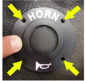
5. Thread the horn button's wire through the 1/8" hole, under the mat and up to the dash area. Place the decal over the button. Mount the decal using the Included Rivets.
