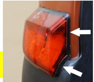
**NOTE:** Do not expose double sided tape until lights are functioning and have been test fit.
