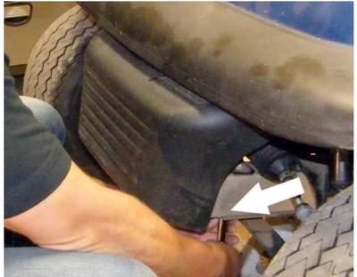
2. On the driver side rear body, measure 2-1/4" over from the vertical body line and 1-1/2" up from the underbody. Mark this location with a center punch. Drill the location with a 1-1/2" hole saw. Sand hole to remove rough edges.
