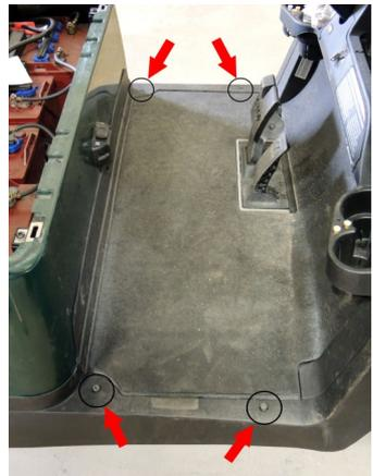
3. Remove the rivet on the pedal group access panel and remove the panel. Retain hardware.
