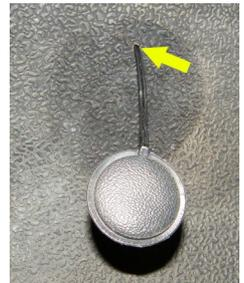
4. Place the horn button decal over the button making sure it is even and the button is centered. Mark the (4) mounting holes. Remove the decal and button. Drill the (4) marked locations with a 3/16" drill bit through the mat ONLY.
