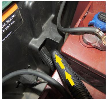
8. Feed the brake light wires through the center floor channel into the pedal group compartment. Use cable ties to secure them to the existing harness.
