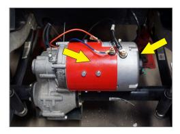
Repeat steps 1 and 2 until the 6-10 mile break-in period is complete and the motor is running cooler.
